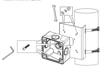
If you are installing a bullet camera directly to the bracket, use the M6 screws in the center. A hex crescent wrench is required.
