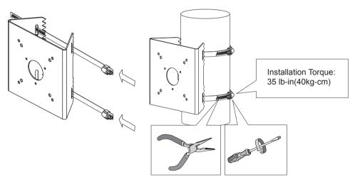
3. The 4 screw holes in the center are used for directly mounting the IB series bullet cameras.
