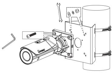
The installation of IB8367A, IB8369A, IB8377, and IB8379 is similar to the above, except using different mounting holes and screws.
